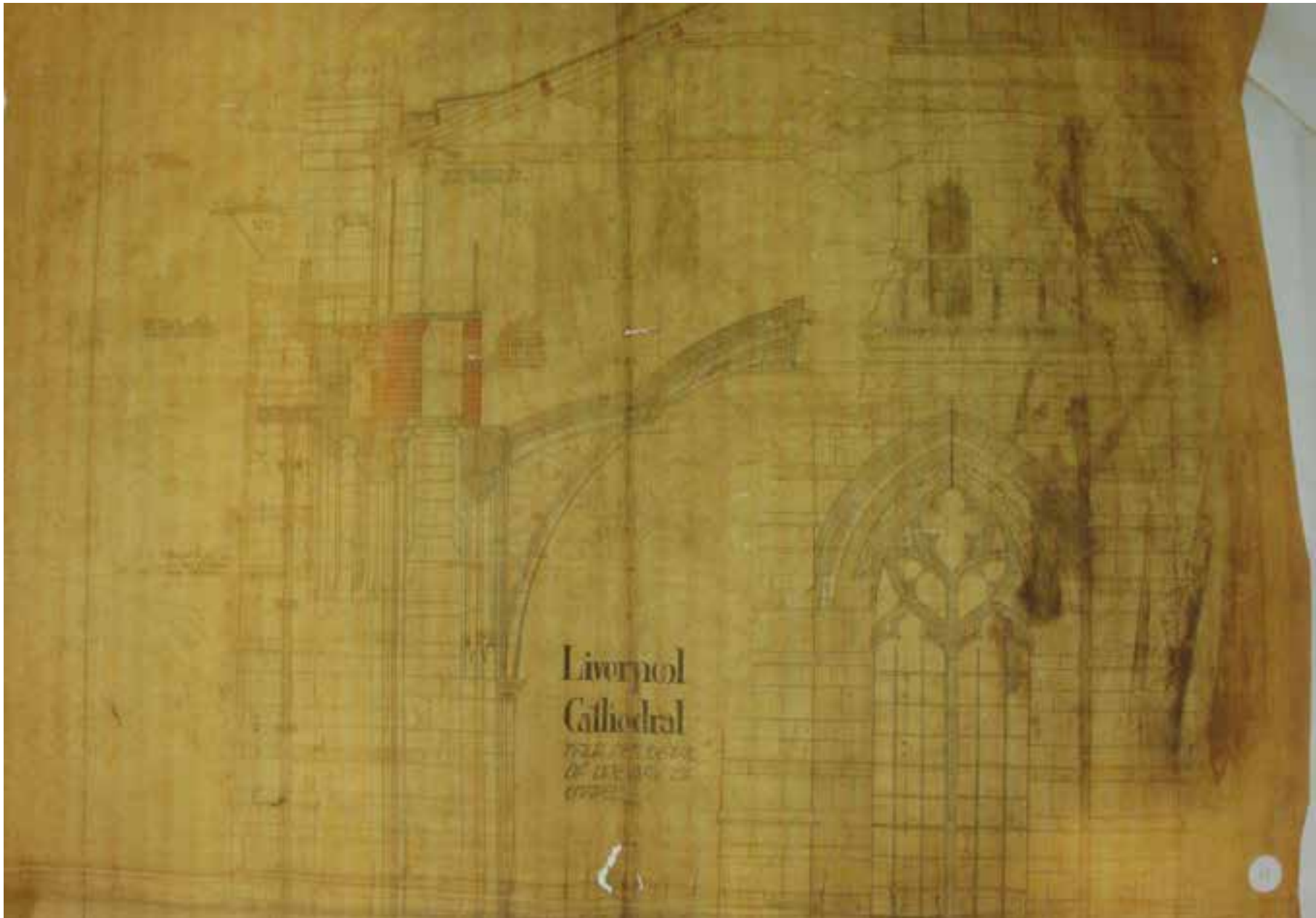
4: Half inch detail of one bay of Lady Chapel, n.d., Liverpool Cathedral Archive, Drawing no. 67)
